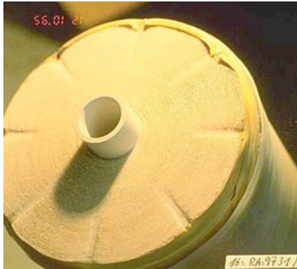
Figure 59: The endcap has been pushed off
